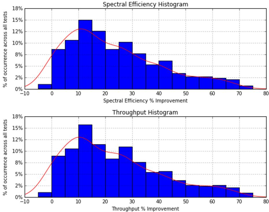
Figure 4.14: Measured spectral efficiency and throughput percentage improvements comparing mode 0 of the modal adaptive antenna system to the three mode system for all field channel conditions for stationary and slow rotating test cases.
