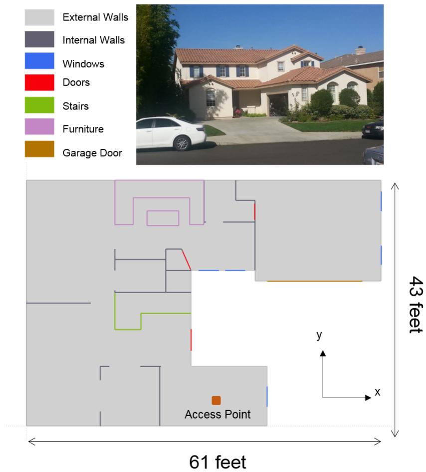
Figure 5.3: First floor layout of the test house including simulation materials.
