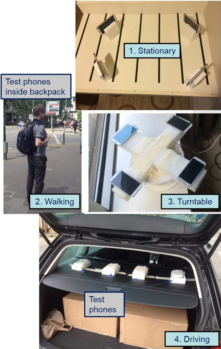
Figure 4.6: Cellular field test use cases (1) stationary, (2) walking, (3) slow rotating turntable (4) driving. In all cases, multiple units are measured simultaneously to increase the sample size of the test and to capture multiple fading channel conditions at the same time.
