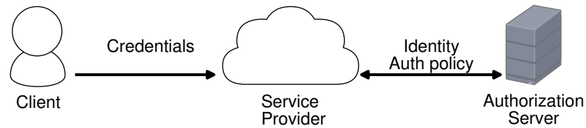
Figure 1.1: The common authorization architecture where a service retrieves authorization policy from a centralized server
