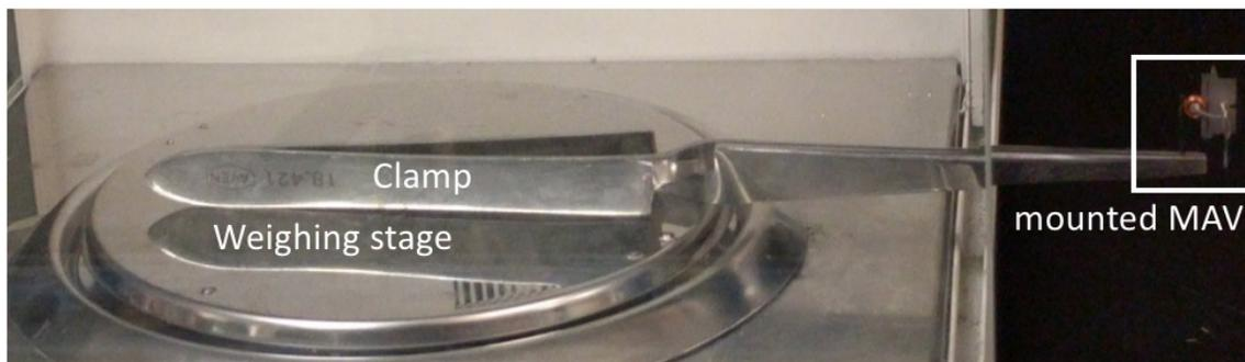
Figure 4.20: Setup for the measurement of average lift.
