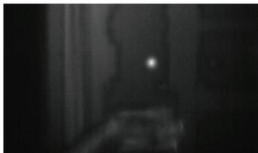
Figure 3.9: Single device light emission test. The uniform circular bright region indicates a uniform electric field distribution and thereby a working device.
