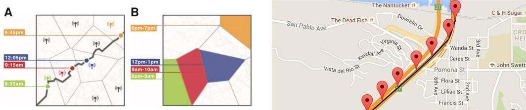
Figure 1.6. Granularity and accuracy L: CDR (from [dHVB13], A shows calls made by users that are received by cell towers, B shows how this cell tower data can be translated into coarse location polygons), R: smartphone app.
