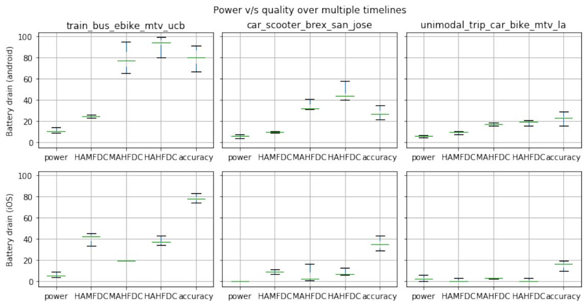
Figure 7.6. **Power drain with different evaluation settings over multiple timelines.** Since we have only three runs each for MAHFDC and HAMFDC, we show the range directly in the plot instead of boxes and outliers. x axis is the battery drain, y axis has a partial order of sensing quality from L  $\rightarrow$  R; MAHFDC and HAMFDC are both medium quality and not comparable. Timelines are from longest to shortest.
