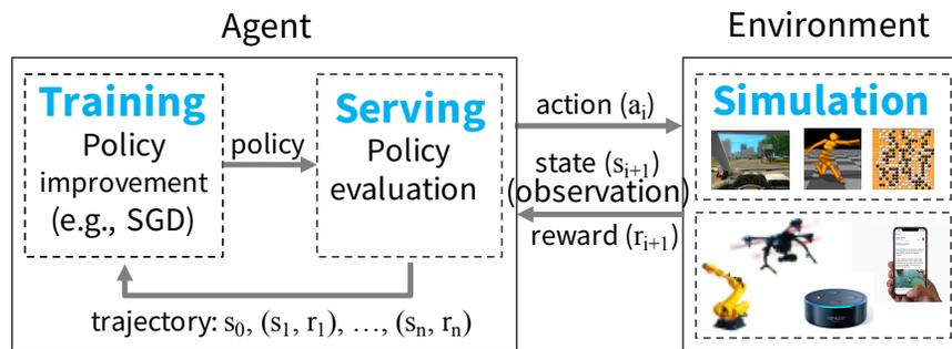
Figure 3.1: Example of an RL system.
