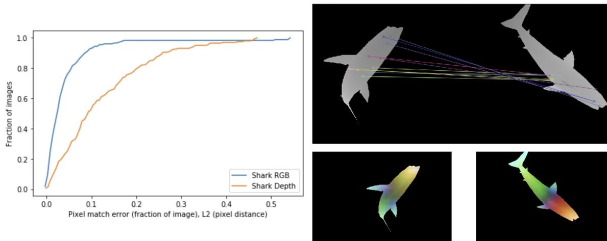
Figure 4.2: Results from applying dense object descriptors to a simulated shark dataset with only depth images. The cumulative distribution plot is shown on the left, and sample images are shown on the right. The top right image shows the best matches between the two images, where points are randomly sampled on the left image and matched with the pixel with the closest corresponding descriptor on the right image. The bottom left images show the mapping of the shark image to descriptor space.
