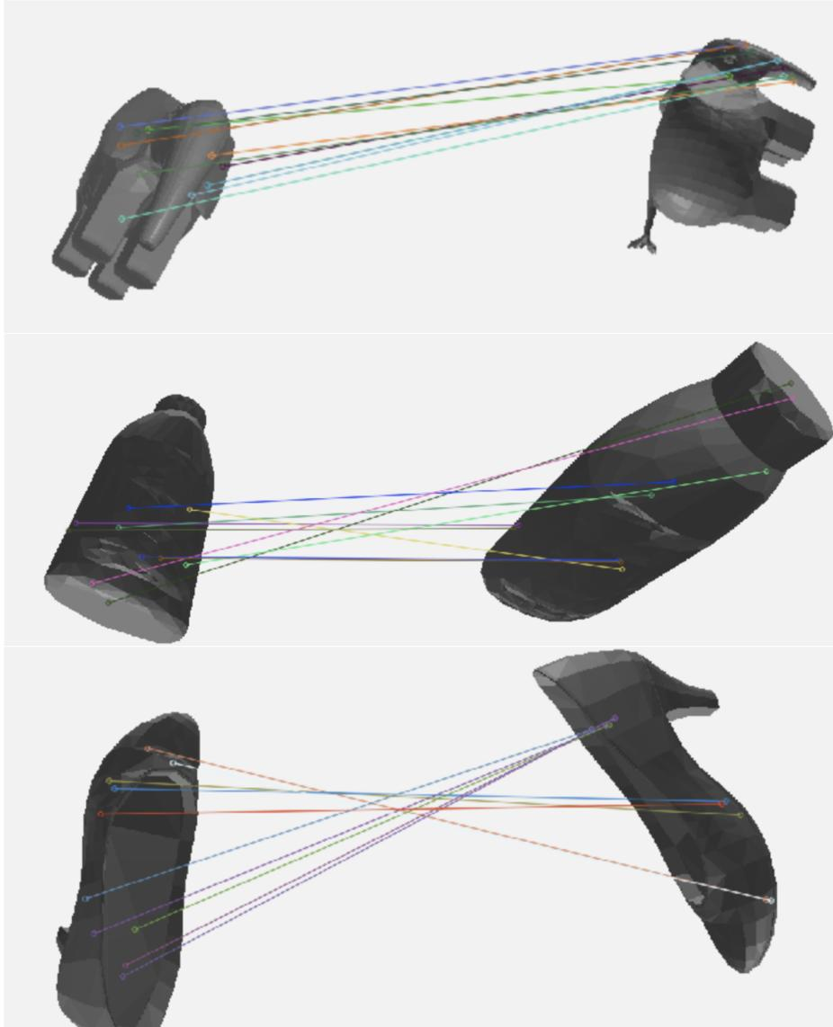
Figure 4.3: Results from applying a network trained on 21 classes on unseen classes. The input to the network is an RGB image, but the images shown are grayscale in order to show the matches between the objects, where points are randomly sampled on the left image and matched with the pixel with the closest corresponding descriptor on the right image.
