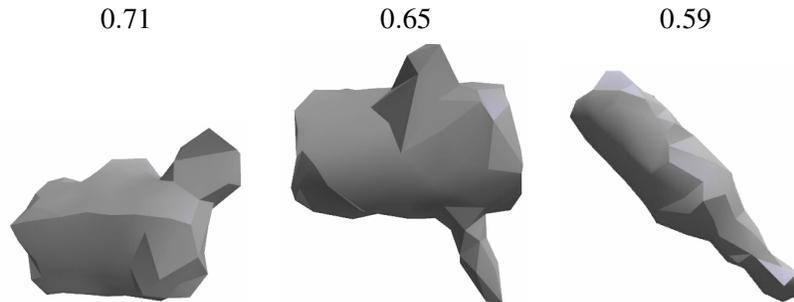
Figure 3.7: Left to right: results after applying the convexity-preserving rejection sampling algorithm to the original objects from Fig. 3.6. The number on top of each object represents the graspability metric for that object
