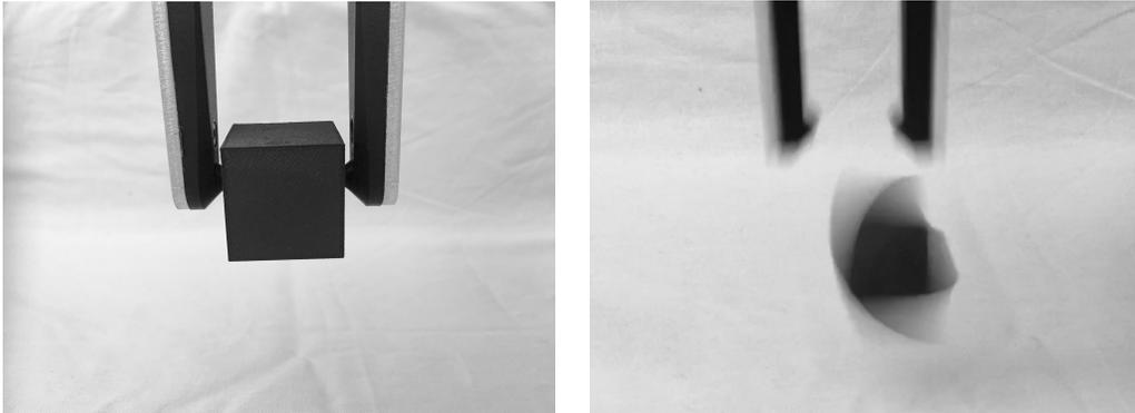
Figure 3.2: Physical experiments on the original and adversarial cubes with a gripper. Both ends of the gripper contain a steel bearing to simulate a point contact. Left: The gripper successfully grasping the original cube. Right: The gripper dropping the adversarial cube.
