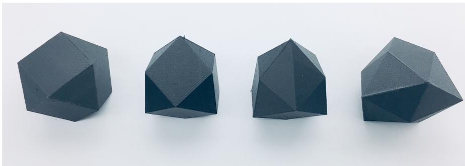
Figure 3.5: 3D printed adversarial cuboctahedrons generated by the convexity-preserving rejection sampling method. Antiespodal threshold from left to right: Original, 10 degrees, 15 degrees, 26 degrees.
