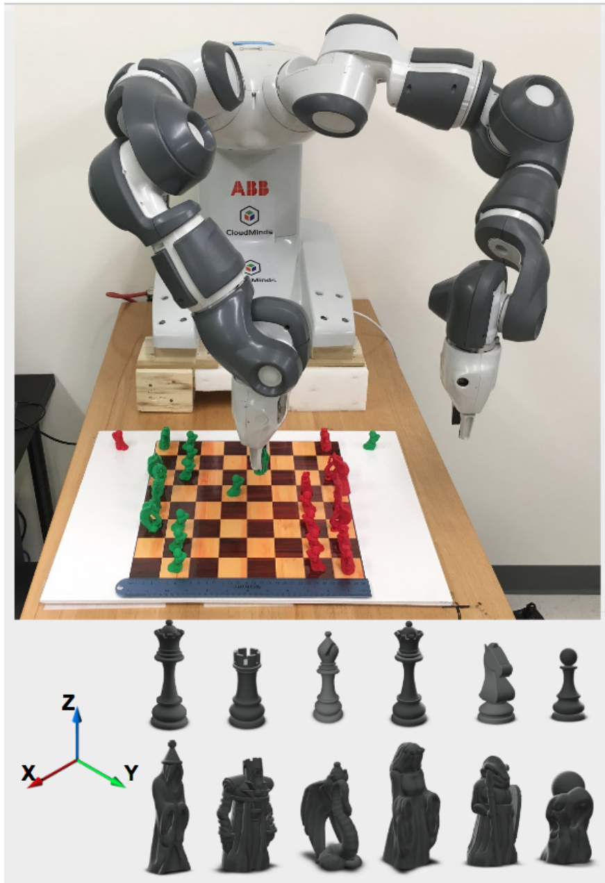
Figure 2.2: Dual-Arm YuMi Robot Playing Non-Standard Chess: (Top) The YuMi robot replaying the classic 1997 chess game where IBM’s Deep Blue defeated world champion Garry Kasparov with asymmetric “wizard” chess pieces (video: https://youtu.be/_LBBX_oxtbA ). (Middle) CAD model of standard chess pieces which can be grasped with hard-coded configurations. (Bottom) CAD model renderings of our non-standard asymmetric chess pieces. The YuMi requires Dex-Net grasp recommendations to manipulate these pieces. The y-axis for each piece points front-to-back, while the x-axis points right-to-left.
