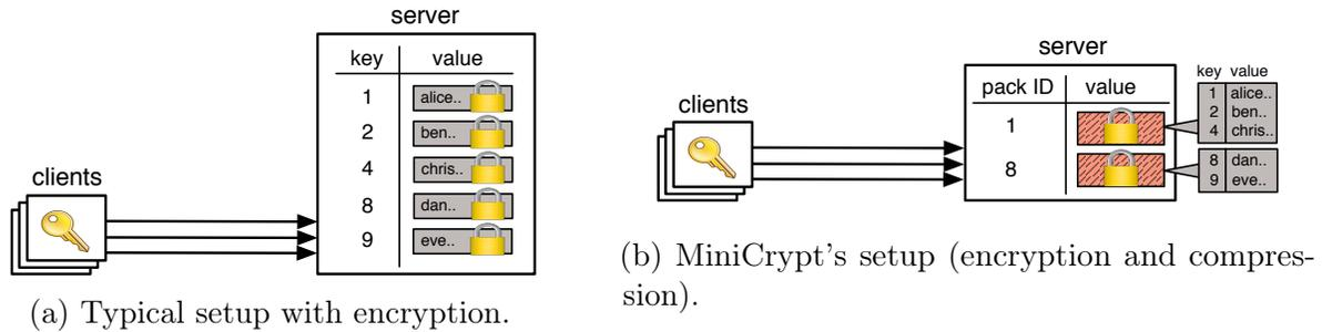
Figure 3.1: System architecture for a typical encrypted key-value store and MiniCrypt. A lock indicates an encrypted item. Orange indicates a compressed item. MiniCrypt's values consist of compressed and encrypted packs.
