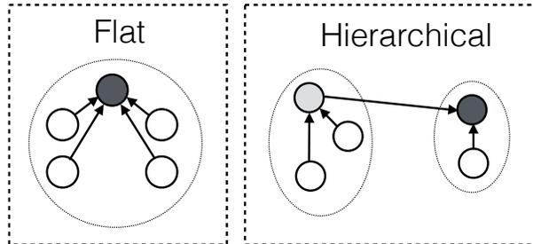
Fig. 6.4: The arrows show the aggregation communication pattern for a single multiplication triple. The shaded nodes represent coordinators.
