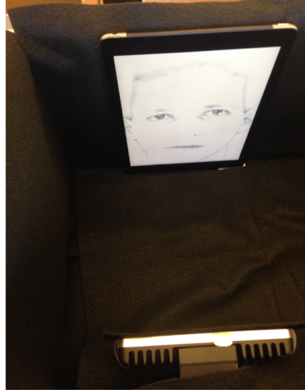
Figure 2.9: Our simplified physical world has a tablet with retina and a fixed webcam in a low-glare box.
