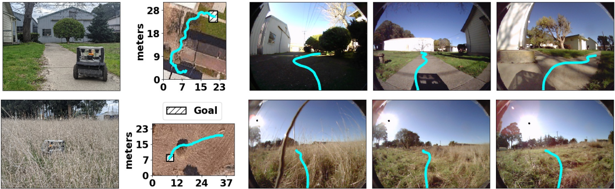
Figure 4.1: BADGR is an end-to-end learning-based mobile robot navigation system that can be trained with self-supervised off-policy data gathered in real-world environments, without any simulation or human supervision. Using only RGB images and GPS, BADGR can follow sparse GPS waypoints without colliding while (top row) preferring smooth concrete paths and (bottom row) ignoring geometrically distracting obstacles such as tall grass.
