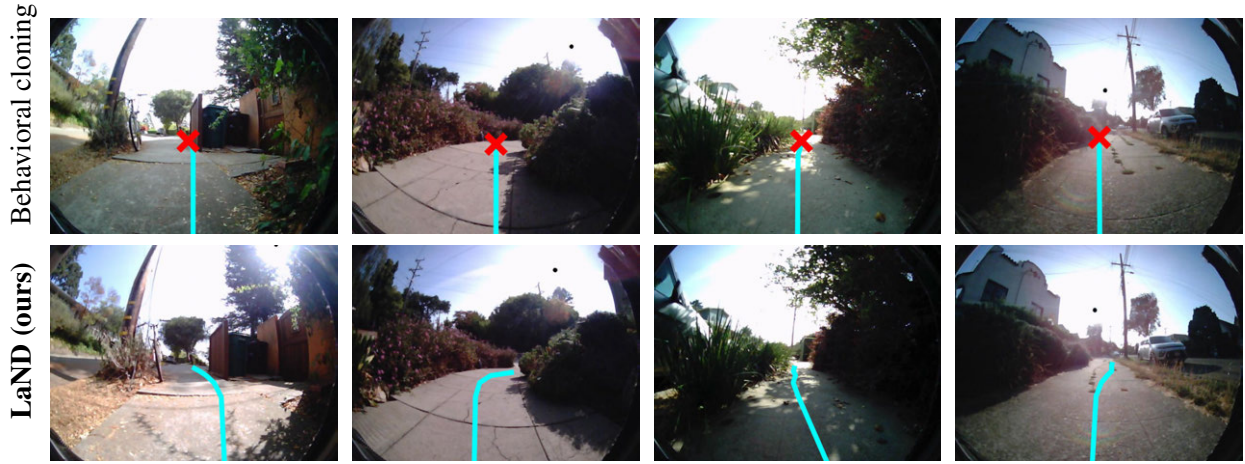
Figure 6.8: Qualitative comparison of our LaND method versus the best performing prior approach (behavioral cloning) in scenarios containing parked bicycles, dense foliage, sun glare, and sharp turns. Our approach successfully navigates these scenarios, while imitation learning is unable to and crashes.
