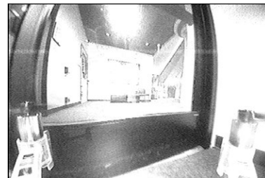
Figure 3.5: Example failure: collision with a glass door.
