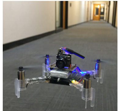
Figure 3.1: Our autonomous quadrotor navigating a building from raw monocular images using a learned collision avoidance policy trained with a simulator and one hour of real-world data.
