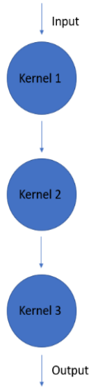
Figure 4: PyPlover Kernel Execution. A kernel chain in our system must process data in a chain (i.e output of previous kernel is input of next kernel)
