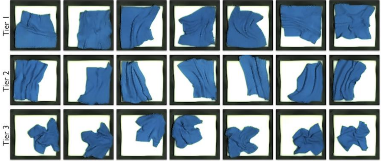
Figure B.4: Representative examples of color images from the physical camera used for the surgical robot experiments, so there is no domain randomization applied here. We manipulated fabrics so that they appeared similar to the simulated states. The color images here correspond to the depth images in Figure B.5.
