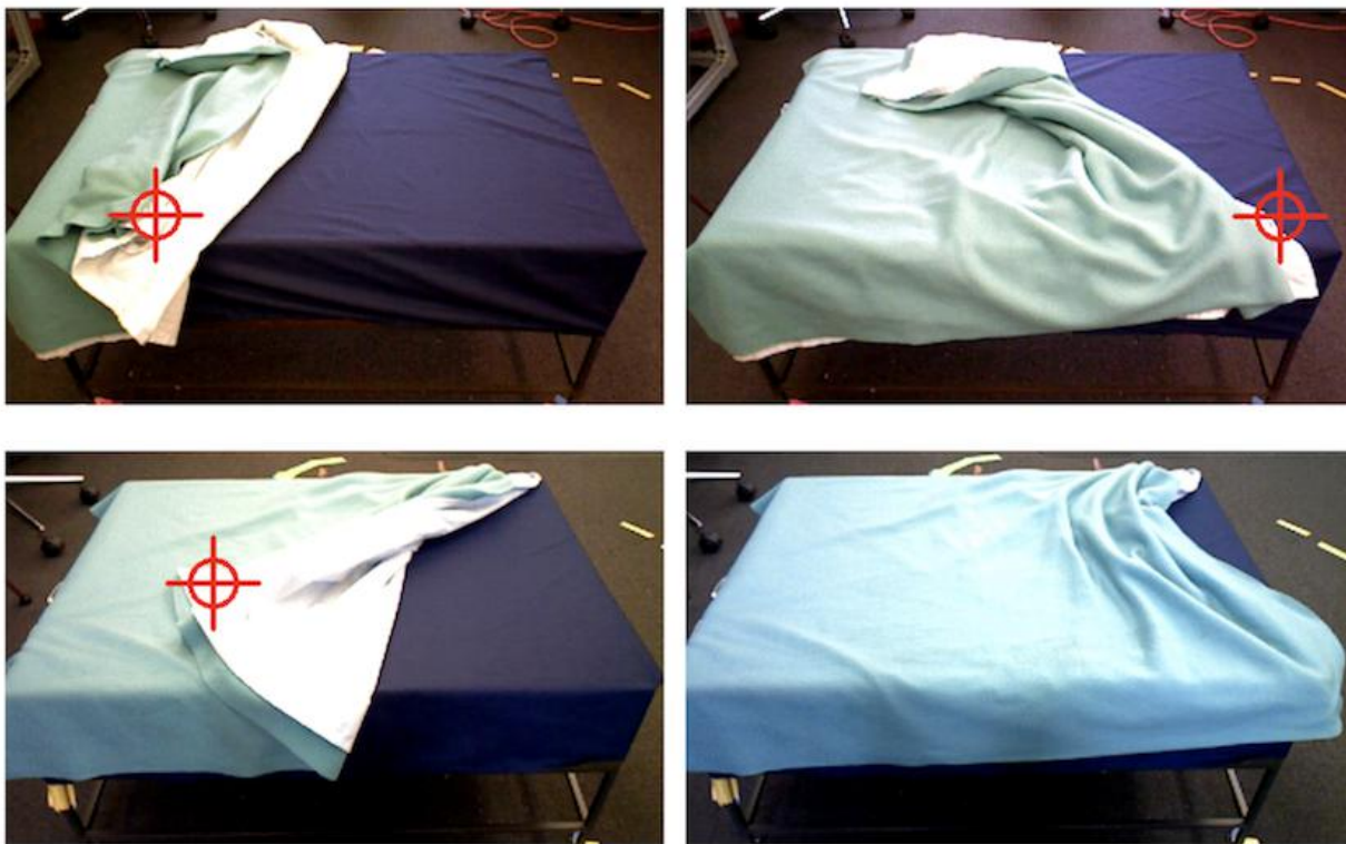
Figure A.2: Two examples of RGB image pairs before and after the robot executes a grasp and pull. Predictions from the grasp network are shown with a red cross hair. Top left: the grasp network suggests a reasonable pick point at the blanket corner, but the robot’s grasp and pull did not pull the blanket all the way due to friction, and furthermore, the corner is slightly off the top of the bed frame. In this case (top right) the robot can still make incremental coverage progress. Bottom row: in a different configuration, the grasp network again picks an excellent pick point (left) and this time, one grasp and pull was enough to cover the side (right).
