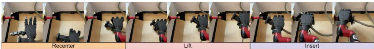
Figure 14.11: Film strip illustrating partial training trajectory of hardware system for pipe insertion. This shows various behaviors encountered during the training - repositioning the object, picking it up, and then inserting it into the wall attachment. As seen here, MTRF is able to successfully learn how to do pipe insertion without any human intervention.
