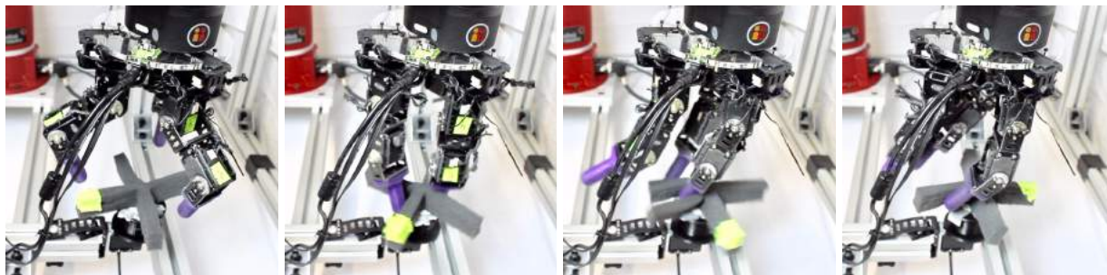
Figure 9.12: DClaw learns to rotate a foam valve despite its deformable structure. The claw learns to focus its manipulation on the center of the valve where there is more rigidity.
