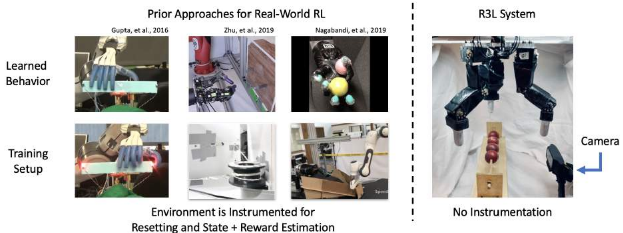
Figure 13.2: We draw a comparison between current real world learning systems which rely on instrumentation versus a system that learns in an environment more representative of the real world, free of instrumentation. While all three prior works utilize instrumentation for resets, state estimation, and reward, the motion capture system of [279], sensor attached to the door in [389], and auxiliary robot which picks up fallen balls in [33] are good examples of engineered state estimation, reward estimation, and reset mechanisms respectively.
