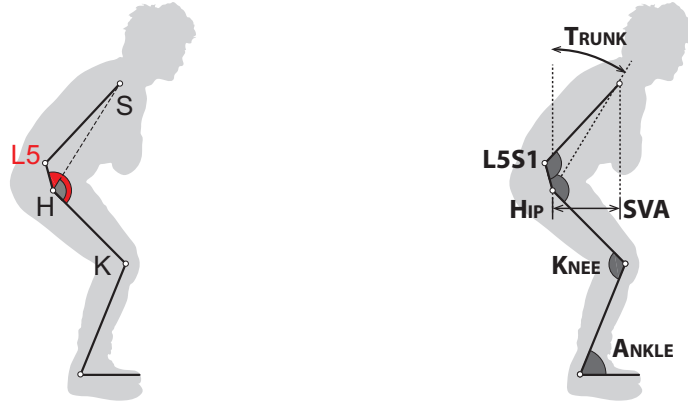
Figure 2.3: Left: Model used for L5S1 angle estimation. The sagittal location of the shoulder, L5S1, hip, and knee are shown. The included angle at the hip is used to predict the angle at L5S1. Right: sagittal plane model. Joint centers and angle definitions are shown. The definition of the Sagittal Vertical Axis (SVA) metric is also shown.
