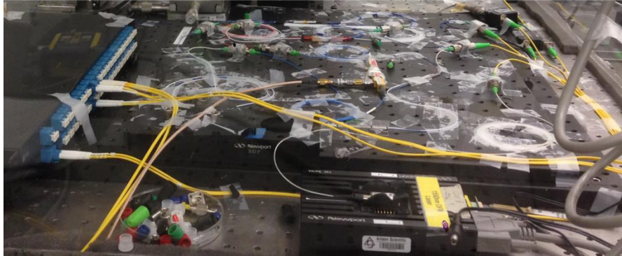
Figure 5.1: a) Schematic of fiber-based interferometry setup. PM is a phase modulator, and DAQ is a data acquisition board. b) A photograph of our fiber-based demultiplexed multiwavelength interferometry setup on a floating optical table. Tapes were used to secure the fibers to the table to stabilize micromovements of the fiber.
