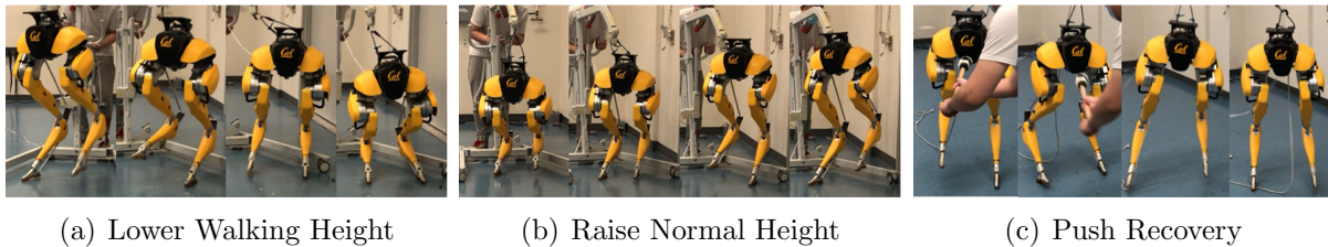
Figure 9.1: Our system is able to learn robust parameterized locomotion controllers for a bipedal Cassie robot. The controller can vary parameters such as walking velocity and height, while also being robust to significant external perturbations. (Video 1 )
