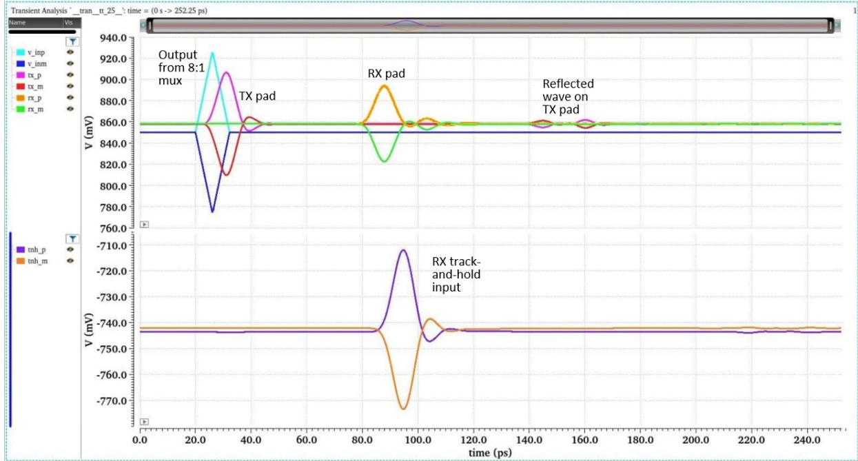
Figure 6.2: Waveforms from Transmitter Output Driver Simulation
