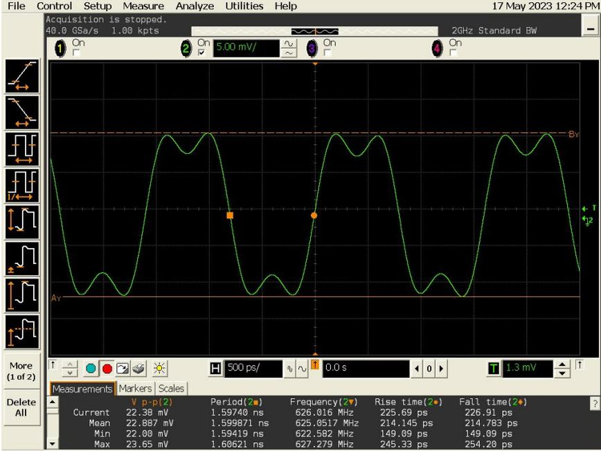
Figure 7.8: Output Divided Clock (10 GHz Injection)
