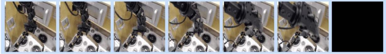
**Figure 51:** Example of unsafe behaviors when running SACfD. The robot collides with the camera during online exploration, resulting in a system crash.
