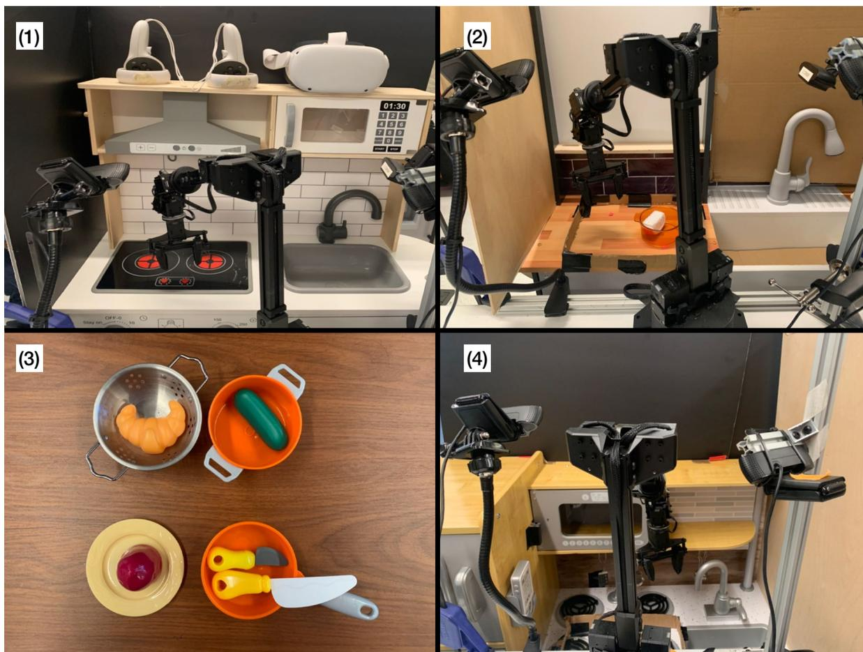
**Figure 43: Setup Overview:** Following Ebert et al. [70], we use a toykitchen setup described in that prior work for our experiments. This utilizes a 6-DoF WidowX 250 robot. **(1):** Held-out toykitchen used for experiments in Scenario 3 (denoted “toykitchen 6”), **(2):** Re-targeting toykitchen used for experiments in Scenario 2 (denoted “toykitchen 2”), **(3):** target objects used in the experiments of scenario 3., **(4):** the held-out kitchen setup used for door opening (“toykitchen 1”).
