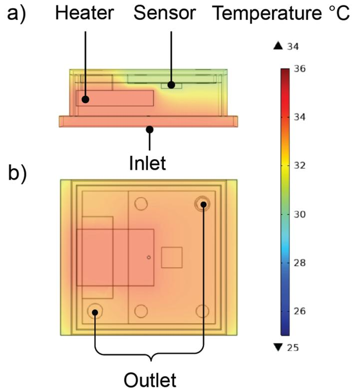
**Figure S2.** Thermal simulation of device worn on-body. Heat distribution within the chamber is shown when ambient, heater and skin temperatures are 25°C, 34°C and 34°C, respectively. a) Side view of a vertical slice through the middle of the device. b) Top view of a horizontal slice through the base of the device, where the Technicloth is placed.
