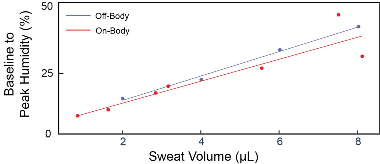
**Figure 7.** The relationship between the baseline-to-peak humidity levels and the volume of liquid injected or secreted for both the on-body and off-body datasets. The red line represents the ordinary least squares line for the on-body dataset (N=7):  $y = 4.1x + 6.9$ ,  $R^2 = 0.83$ . The blue line represents the ordinary least squares line for the off-body dataset (N=4) as presented in Fig. 4d:  $y = 4.5x + 6.9$ ,  $R^2 = 0.99$ .
