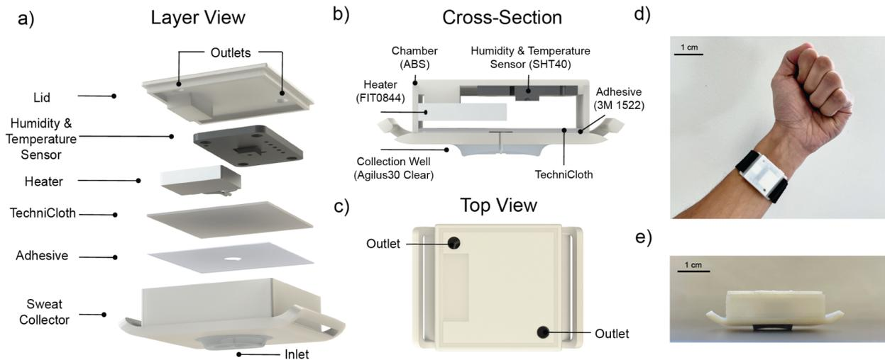
**Figure 1.** Wearable device to monitor sweat rate from the change in sweat-induced humidity levels. a) Layer-by-layer stack of the device structure and its components including a humidity and temperature sensor, a microheater, a Technicloth layer, double-sided adhesive, and the sweat collector. b) A cross-sectional schematic of the device when assembled and the materials used for each component. c) A top view of the device, showing the lid's two ventilation holes. d) The
