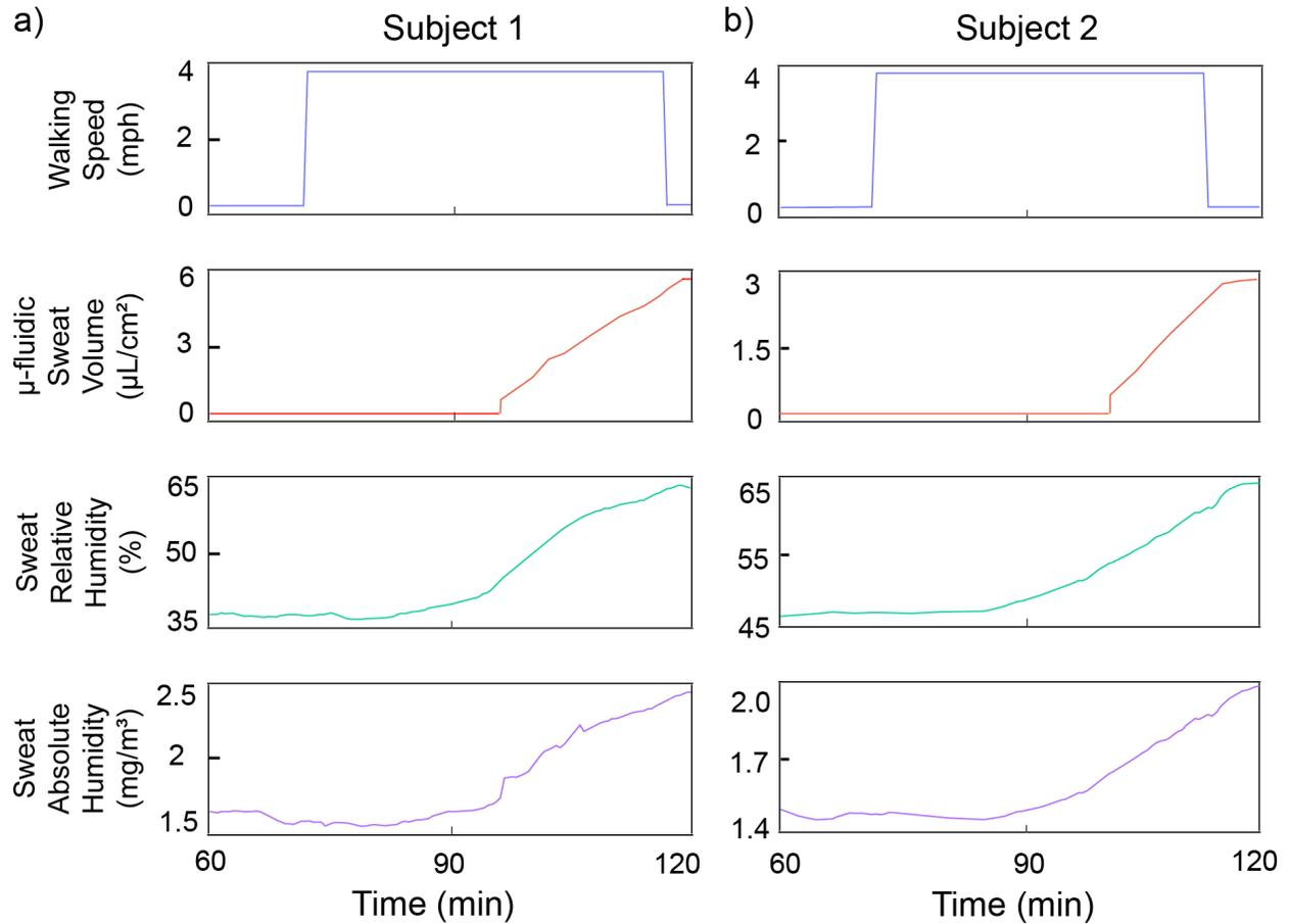
**Figure S4.** The results from two experiments where two unique subjects performed the same exercise of walking at 4 mph for 45 minutes. a-b) The microfluidic sweat volume was recorded using a microfluidic device and the chamber relative humidity was recorded from the device presented in this paper. The absolute humidity plot is shown to highlight the trend similarity between relative humidity and absolute humidity when chamber temperature fluctuations are minimal.
