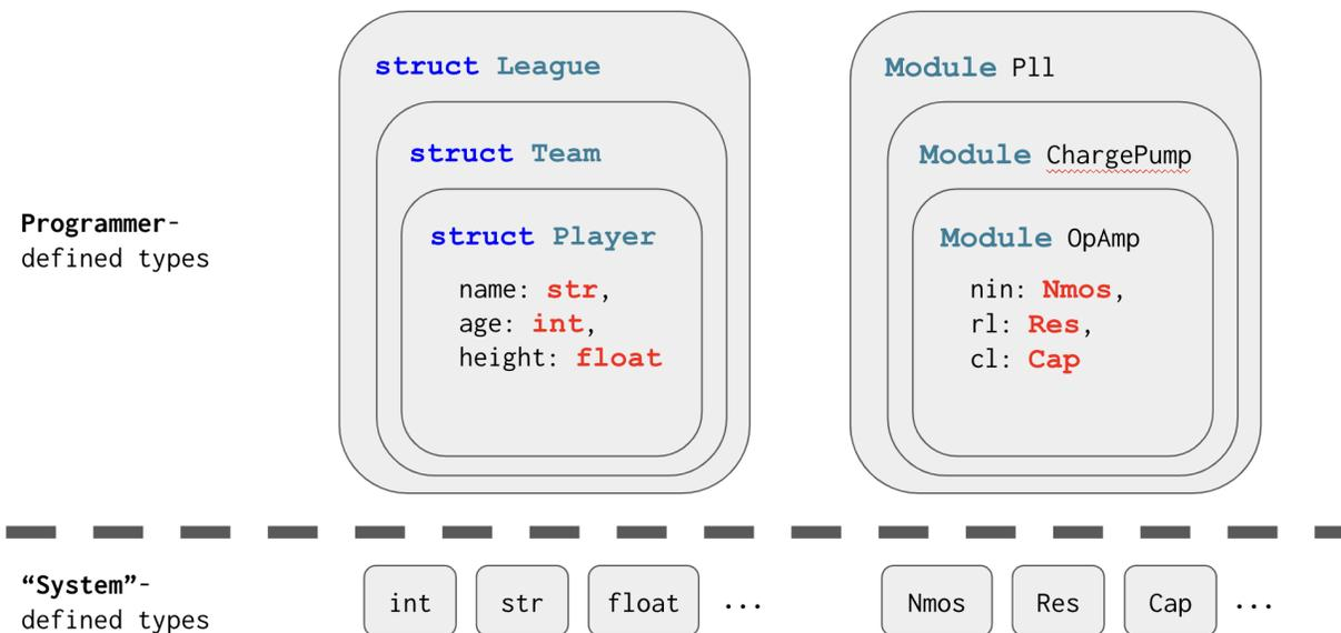
Figure 3.1: Primitives in a Typical Programming Language, and in Hdl21
