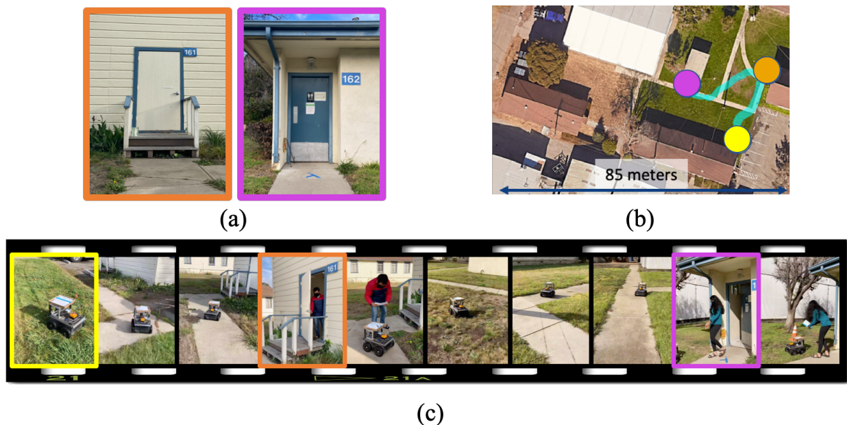
Figure 8: Contactless Last-Mile Delivery Demo: Given a set of visually-indicated goals (a), ViNG can perform contactless delivery in the urban neighborhood successfully, as shown in the filmstrip (c). An overhead view (b) with starting position marked in yellow and respective goals marked in orange and magenta shows the trajectory of the robot (cyan). Note: The satellite view (b) is solely for visualization and is not available to the robot.
