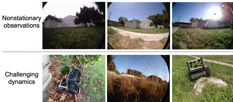
Figure 2: Challenges with Real-World Navigation: (Top) Three observations taken from exactly the same position at different times of day exhibit large differences. (Bottom) While tall grass and inclined rocks are traversable, a hole filled with dry leaves is not. These examples highlight the challenges with geometric reasoning about traversability.
