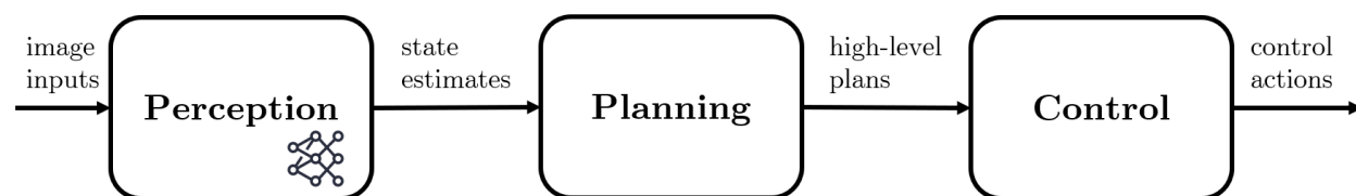
Figure 1.1: An example perception-planning-control pipeline for vision-based navigation. Neural network icon by dmitrychae.
