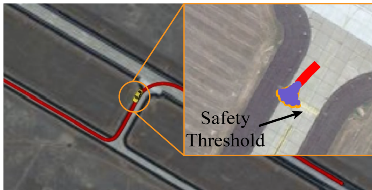
Figure 2.4: Our algorithm is applied to assure safety in potential runway incursion scenarios. Once the ground vehicle is determined to have crossed a designated safety threshold, the aircraft is cleared to land. most-likely GMM mode. In Figure 2.3b and Figure 2.3c, we can visually discern the benefit of including these features.
