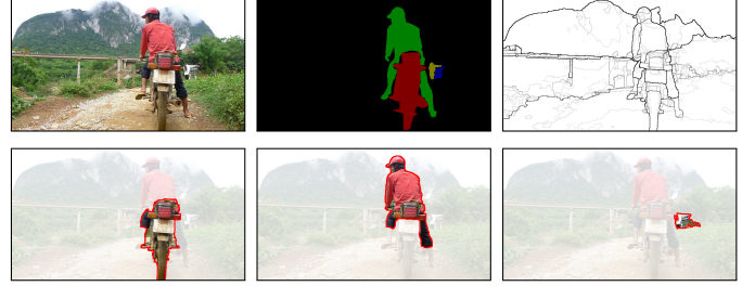
Fig. 1. Top: original image, instance-level ground truth from COCO and our multiscale hierarchical segmentation. Bottom: our best object proposals among 150.
