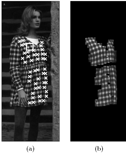
Fig. 2. A textile image on a curved surface. The rectangle in (a) is the initial unit we found. The crosses are the locations of the units grouped together. In (b), the segmented region is shown. Notice that the rectangle includes two units in the actual pattern. This is due to the inherent ambiguity in defining a repeating unit, namely, 2 units together is still a repeating element.
