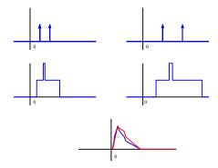
Figure 3: Top row: A signal and a dilated version of the signal. Second Row: Geometric blur of both signals. Bottom: Red line is comparison over varying dilation using  $\tilde{C}$ , Blue line (lower) is comparison using  $\hat{C}$ . The peak is at no dilation and the falloff of both is close to linear in the change in dilation.
