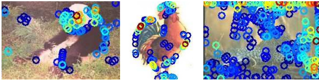
Figure 3.9: Visualizations of the weights learned by our algorithm for one type of shape feature (geometric blur with 42-pixel radius) for three images from our training set. Each circle is centered at the center point of the feature’s patch and the color of the circle indicates the relative value of the weight. The colors are on Matlab’s jet scale, where dark red is the highest weight (most salient feature) and dark blue is the lowest non-zero weight. Weights that were assigned a zero weight are not shown. For (a), the algorithm learned zero weights for all but 83 of the 400 small geometric blur features computed for the image, and learned that the most important feature is the patch around the eye of the panda. For (b) it learned that the most useful features are on the breast and tail of the rooster, and assigned zero weights to all but 79 of the roughly 400 small geometric blur features. For (c) it learned that the best features aren’t on the leopard at all, but are along the right edge and in the upper-right corner of the image. The Leopards images were drawn from the Corel image set and they have a thin black border around the image that algorithms can exploit, making it a surprisingly easy category.
