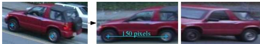
Figure 2: Detecting and warping car images into alignment: Our identification algorithm assumes that a detection process has found members of the class and approximately aligned them to a canonical view. For our data set, detection is performed by a blob tracker. A projective warp to align the sides is computed by calibrating the pose of the camera to the road and finding the wheels of the vehicle. Note that this is only a rough approximation (the two warped images, center and right, are far from perfectly aligned) that helps to simplify our patch descriptors and positional bookkeeping.
